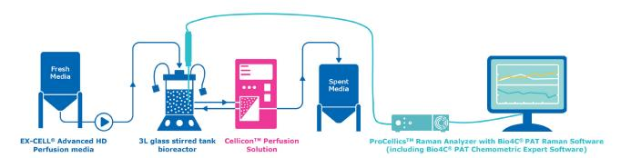
Figure 1: Set up of a perfusion cell culture monitored with ProCellics™ Raman Analyzer
