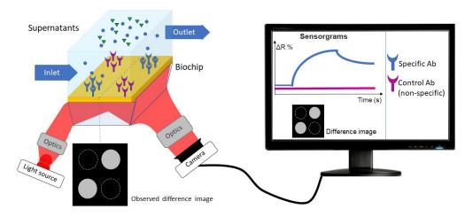
Figure 1: Schematic representation of the multiplexed detection of selected biomarkers via Surface Plasmon Resonance imaging (SPRi)
