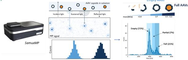
Figure 1: Principle of Mass photometry (Part of the figure was provided by Refeyn)
