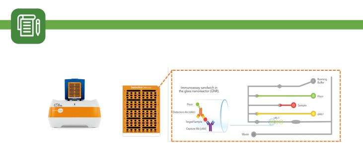
**Figure 2. ELLA Equipment and its cartridge.** Each sample well Assays are carried out within Glass Nano Reactors (GNRs), which are coated with analyte specific capture antibodies. GNRs and other assay reagents come preassembled into the microfluidic circuitry of the Simple Plex cartridge. Setting up a run simply requires loading the cartridge with diluted and centrifuged samples and wash buffer. Once a run is initiated, Ella automates every step of the assay in less than 90 minutes.
